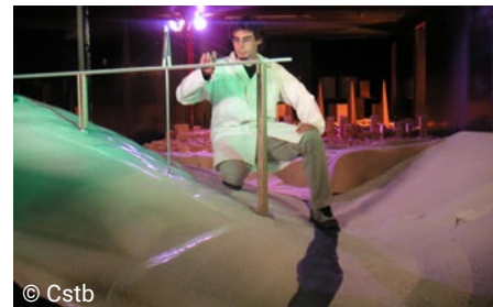
Aeroelastic model of a construction stage
