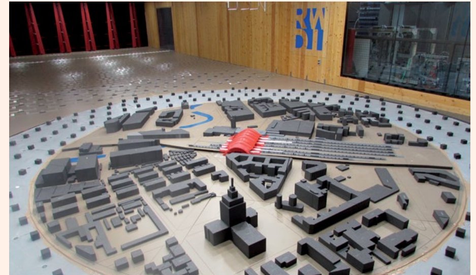
Riga station model in RWDI wind tunnel Lab
