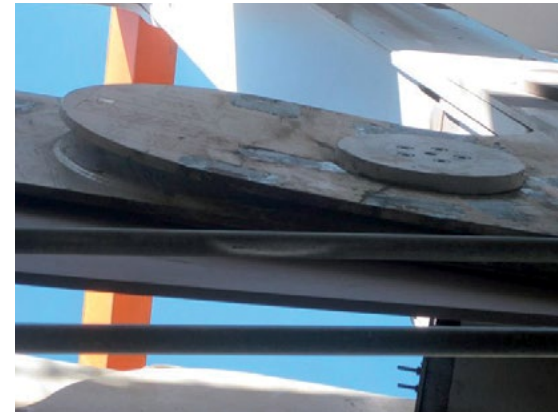
Plastification pattern in the cover plate
