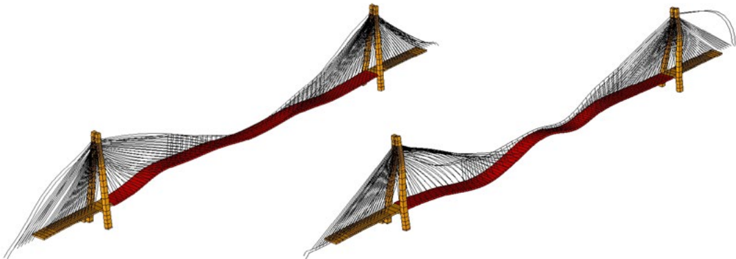
Deformed shapes during earthquake.
